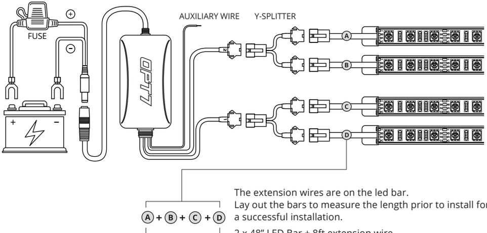
The extension wires are on the led bar.
