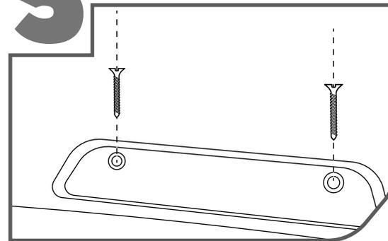
Install the 2 fasteners that were removed from the original brake light housing.
