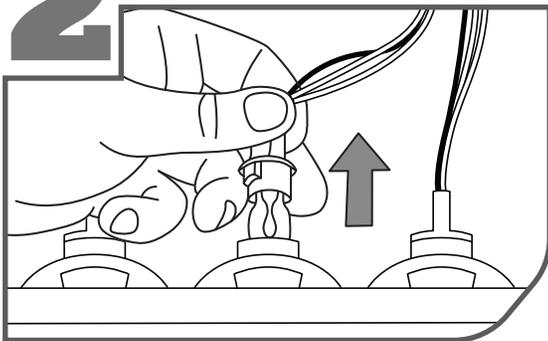
1. Remove bulb socket from original 3rd brake light housing.
