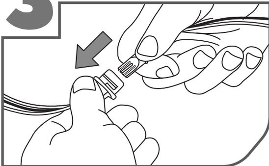
1. Insert Red/Black wire connector from OPT7 light housing into one of the original "Brake light" bulb socket. Leave the other "Brake light" bulb socket empty.
