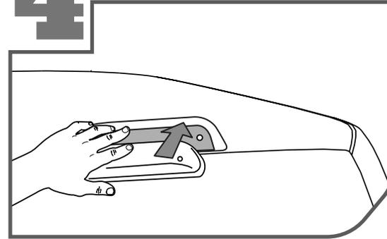
Seat the new brake light housing into it's appropriate slot.
