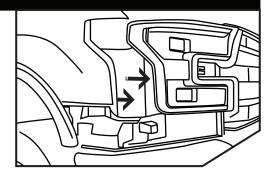
Pull the front of the projector headlight towards you to remove the headlight housing from the vehicle.
