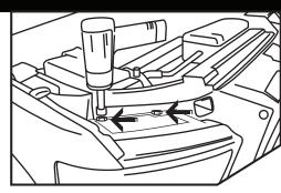
Remove the two bolts on top of the headlight housing using the screwdriver.
