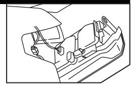
Unplug the electrical harness from the back of the headlight housing.
