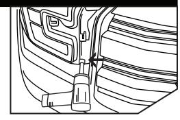
Replace the bolt to secure the headlight.
