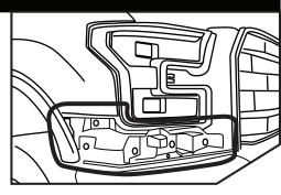
Remove the bolts holding the plastic reinforcement.
