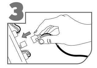
Connect the electrical plug to your new brake light housing.
