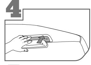
Seat the new brake light housing into it's appropriate slot.
