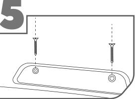
Install the 2 fasteners that were removed from the original brake light housing.
