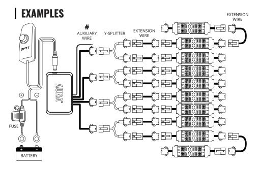
We provide multiple sets of extension wires for you to configure. You can quickly extend them wherever you want to install.
