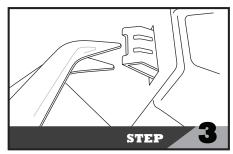
Remove the front grille by releasing (6x) retaining clips.
