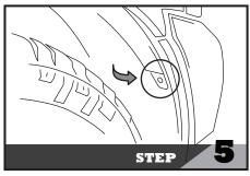
Remove the 10mm bolt (1x) to open the fender liner.
