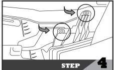
Remove the 10mm bolts (2x) from the OEM headlight as shown in step 4.
