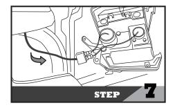
Release the OEM headlight and disconnect the headlight harness.
