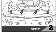
Remove the 10mm bolts(4x) from the grille as shown in step 2.
