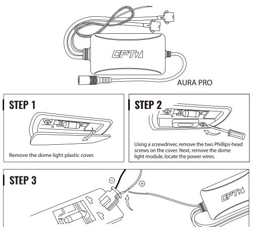
Connect AUX wire to the positive wire on the Dome light.
