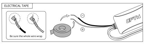
Using the electrical tape method, take two pieces of tape and carefully wrap them fully if you do not wish to use the DOOR ASSIST/AUX wires at all in the near future. Ensure to move the wires away from any positive power source that may trigger them on.
