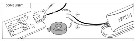
If you plan to not use the DOOR ASSIST/AUX Wires, simply use a good amount of electrical tape to wrap the (+) very carefully, next connect the (-) wire to the negative dome light. This will fix any flashing white light issues that may occur if these wires are left unconnected.
