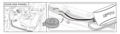
You can use a pry tool to remove the plastic cover on the side door panel. Afterward, connect the "-" wire to a negative power source. Make sure to tap into the wires safely. If you're not familiar with this process, it's advisable to seek assistance from a professional.
