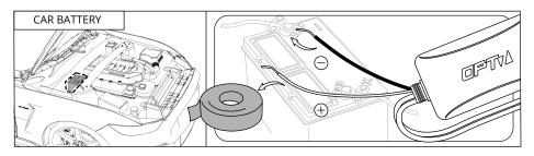
Most AURA kits if installing near the engine bay, you may also connect the following to the car's battery. Simply take the (-) terminal to the (-) battery terminal, and using the electrical tape method to wrap the (+) wire on the control box.
