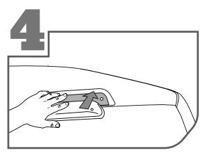
Seat the new brake light housing into it's appropriate slot.
