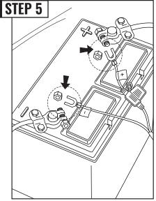
Connect the power wire harness to your vehicle battery.
