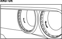
Attach the strip as pictured as an alternate method of install.
