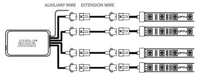
Once connected, plug the control box Cigarette Power Adapter into an available 12 volt charging port.
