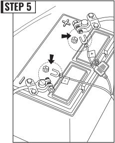
Connect the power wire harness to your vehicle battery.
