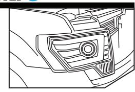
Line up the headlight housing mounting tabs and push rearward to seat it in place.
