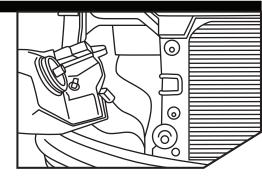
Reattach the electrical connectors to the new headlight housing.
