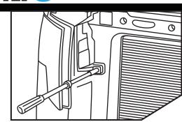
Remove the last bolt retaining the headlight.
