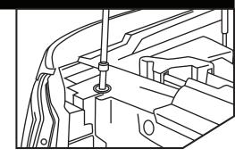
Remove the 2 bolts on top of the headlight.
