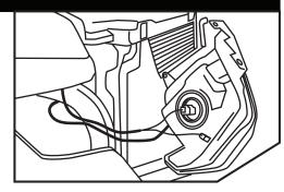
Unclip the electrical connectors on the back of the headlight housing.
